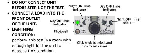
NOTE: read ON times on the LEFT scale and OFF times on the RIGHT scale.
