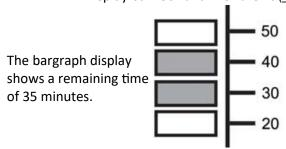
NIGHT is detected and **OFF time** will run for 35 more minutes before it switches to ON time.
