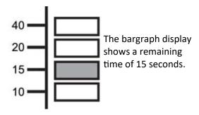
DAY is detected and **ON time** will run for 15 more seconds before it switches to OFF time.
