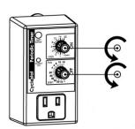
**B.** Within 5 seconds, plug in the unit then set both values to maximum.
